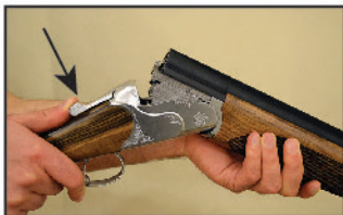
1- Opening your shotgun by pushing the top lever to the right while pushing the barrel downward.
