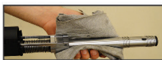
7- Push the latch under the trigger group (Loading figure 2/cartridge drop lever). Pull back the bolt handle. Clean the outer surface of magazine tube with a soft cloth.
