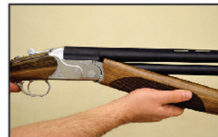
7- Mount the forearm to the barrel as seen in the figure. Be sure the opening latch of forearm is completely closed.
