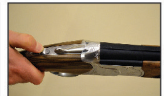
8- Put the safety on by moving the safety switch to the rear position.
