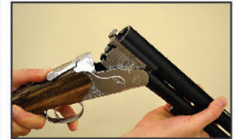
4- While keeping the top lever pushed to right install the barrel to the receiver with an approx 40 - degree angel as it is seen in the figure. Be sure the barrel is completely installed to the receiver otherwise shotgun will not close.
