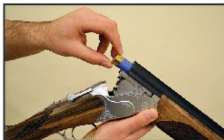
2- MAKE SURE THE SAFETY IS ON. (Moved to rear "S" exposed) Install the suitable cartridges according to your shotgun's gauge and chamber length.
