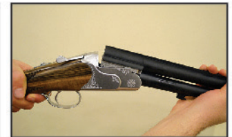
6- By forcing the barrel upwards close the shotgun, be sure the barrel and receiver are properly aligned and top lever returns to slightly to the right of center. It is normal that the top lever does not return exactly to the center, this allows for wear.
