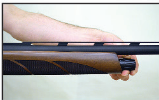
1- Unscrew the magazine cap.
