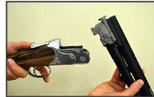
3- Push the top lever fully to the right.
