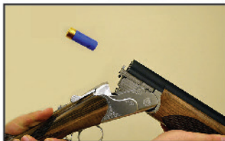
6- After shooting open the shotgun by pushing the top lever fully to the right. Fired cartridges will be lifted for easy removal or ejected if your gun is fitted with automatic ejectors.
